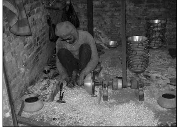
**Fig 2:** Grinding and polishing of metal.
