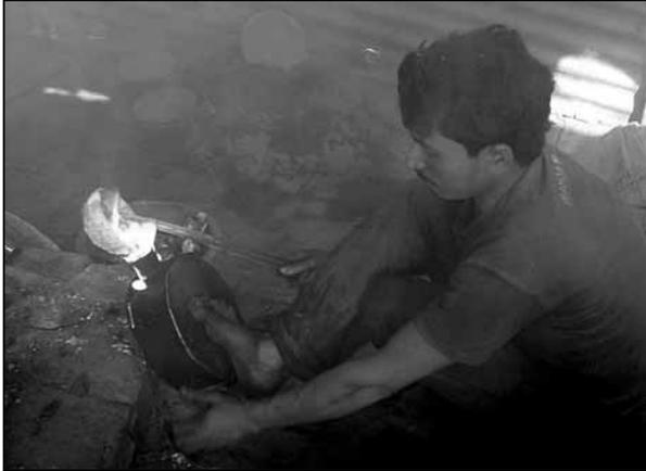
**Fig 1:** Metal casting work without protection.
